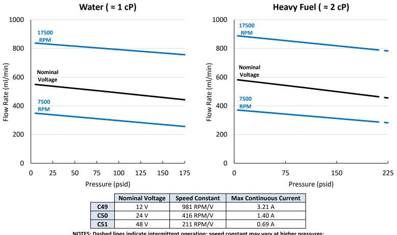
NOTES: Dashed lines indicate <u>intermittent</u> operation; speed constant may vary at higher pressures; RPM flow lines indicate performance at typical maximum and minimum speeds;
